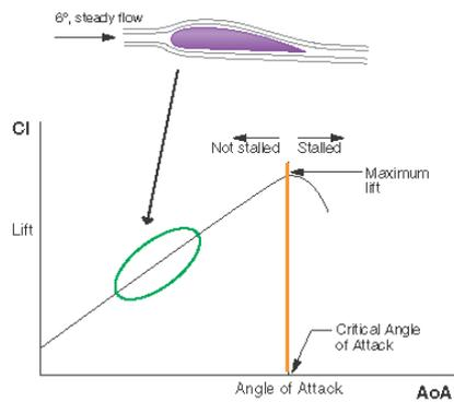
Beyond this point, the lift decreases as the flow is separated from the wing profile. The wing is stalled.
