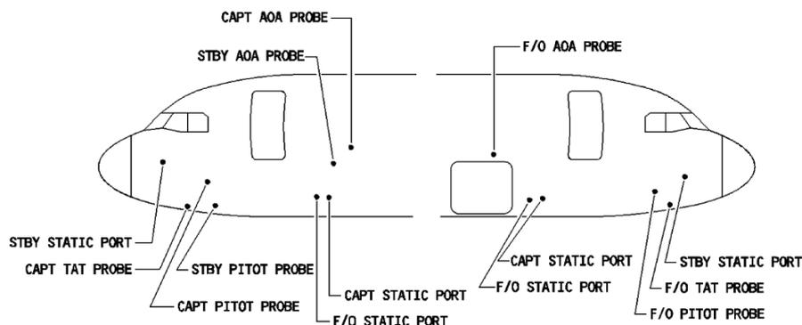
Figure 12: The Pitot Static Configuration
