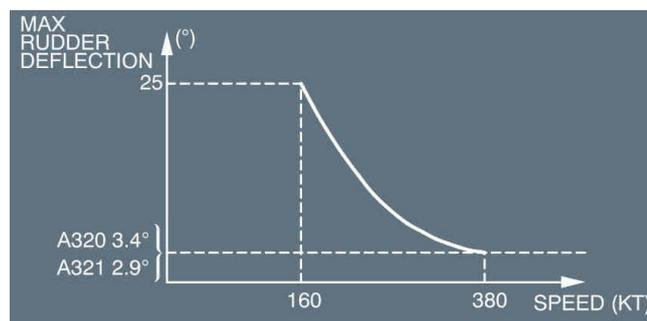
If both FACs lose the rudder travel limitation function, the value of the rudder deflection limit is locked at the time of the second failure.
