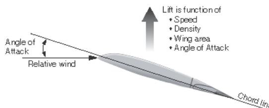
The lift coefficient increases as a function of the Angle of Attack (AoA) up to a value, called Maximum lift, where it starts to decrease.
